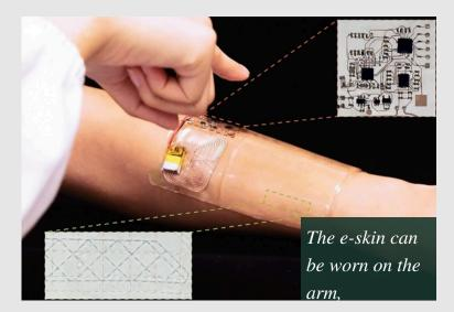
polydimethylsiloxane a silicon-based polymer that is commonly used in biomedical applications. The biogel layers receive their ability to transmit and receive electrical signals from a pattern of microchannels on their surface. The end result is a sensor that is thin, flexible, soft, stretchable, and transparent. These features make it suitable for a wide range of applications where an object-sensing system needs to conform to an irregular surface, like the human body.
